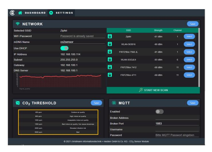
The Sensor shows its IP address on the screen upon rebooting. Now the web interface can be accessed inside the local network it was connected to.
